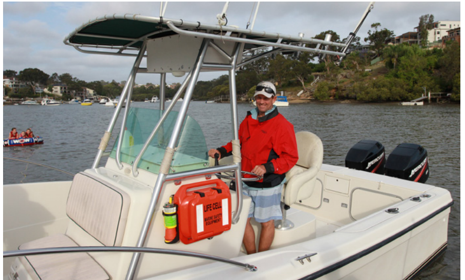
The Life Cell is designed to float free of its bracket if the vessel sinks too fast for someone to grab it.
