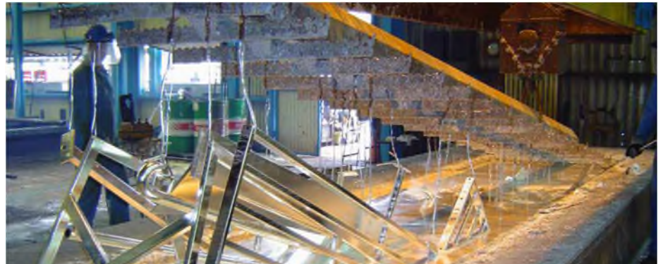
Hot dip galvanizing process
