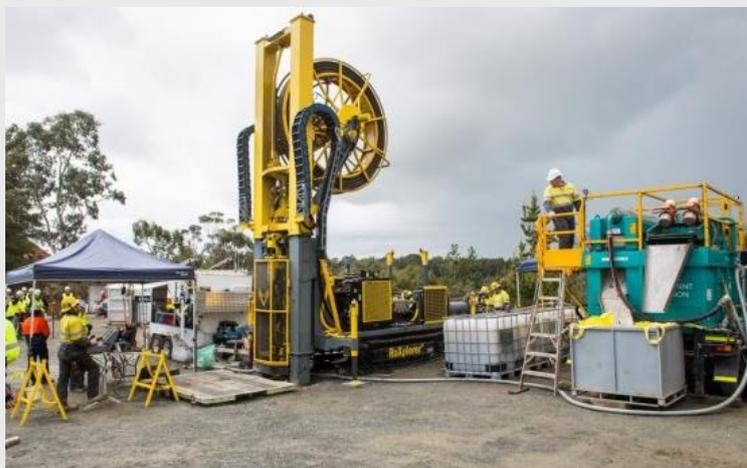
The RoXplorer® rig is small and lightweight. It has a small drill pad, fluid recycling, and lower consumables (e.g. fuel). This means coiled tubing drilling has a lower environmental impact than conventional drilling methods.
